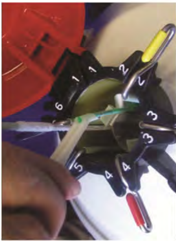
A) Taking the straw out the liquid nitrogen tank while the canister is kept down in the liquid nitrogen to avoid rising the temperature of the straws
