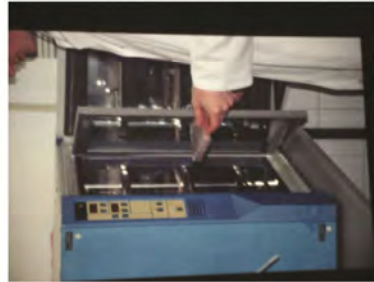
F) Putting the plate in a CO 2 incubator at 39 °C for 24h
