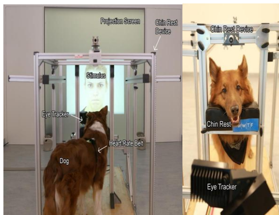
Figure 1. The experimental set up. Left: view from the rear of the room with prospect on the chin rest and the projection screen. Right: front view on the chin rest with prospect on the eye tracker
